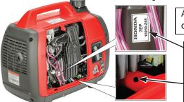
A "green dot" located on the carton. A "7EP" label on the engine cover OR A black dot on the side cover boss.
