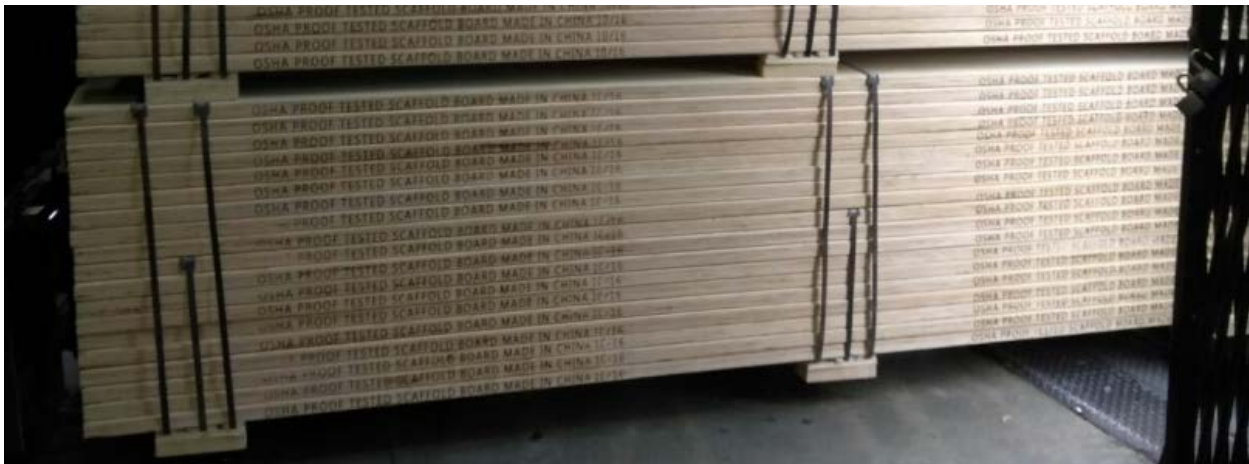
Picture 1: Units of LVL Plank missing identification of product, manufacturer or third-party inspection agency.
